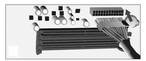
Connect the 8-pin or 4+4-pin connector for the CPU. If your motherboard has an 8-pin socket with a cover on some of the openings, we recommend that you remove the cover and use the 8-pin connector.
